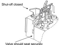
Engage the valve and depress the latch pin. Do not force or you could bend the pin. If you have difficulty, remount the valve and try again. Be sure the valve base is completely seated against the block. Open the shut-off valves by turning 1/4 turn (arrows pointed toward service line) to engage system pressure.
