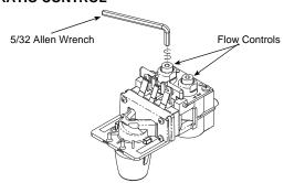
You will need a syrup separator, hex wrench (5/32 Allen), and brix cup. Place the Flomatic S-tube syrup separator (part no.1089-00) over the syrup diffuser. You need not remove the nozzle.
