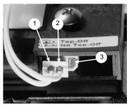
The Automatic Fill valve requires no sensitivity adjustments. The valve automatically delays top-off if more foam is present after the initial pour, and performs a top-off more quickly if less foam is present.
